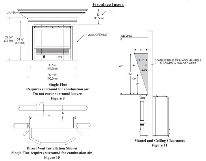
**Note:** The Mantis Power-Vent High-Efficiency Fireplace has been tested and approved for zero clearance to combustible materials. Empire Comfort Systems, Inc. recommends that clearances as listed above should be maintained to allow for removal of the product for servicing.
